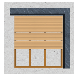
Diagonal installation substructure; 250mm on center maximum joists. More severe angles may require closer joist spacing.
